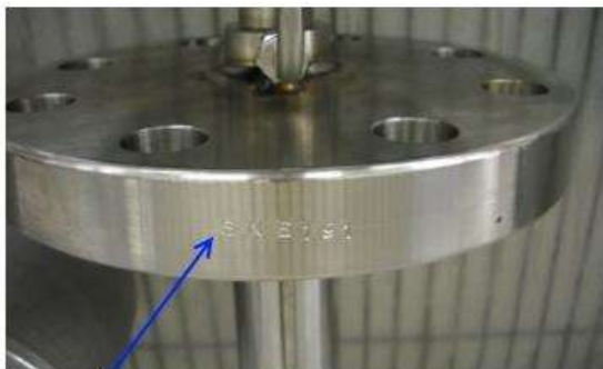
Insertion units stamped at the flange
